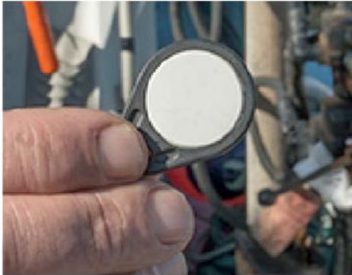
Figure 12: The quarter-size RFID tag used for crab pots by Quinault Indian Nation (NWIFC, 2015).
